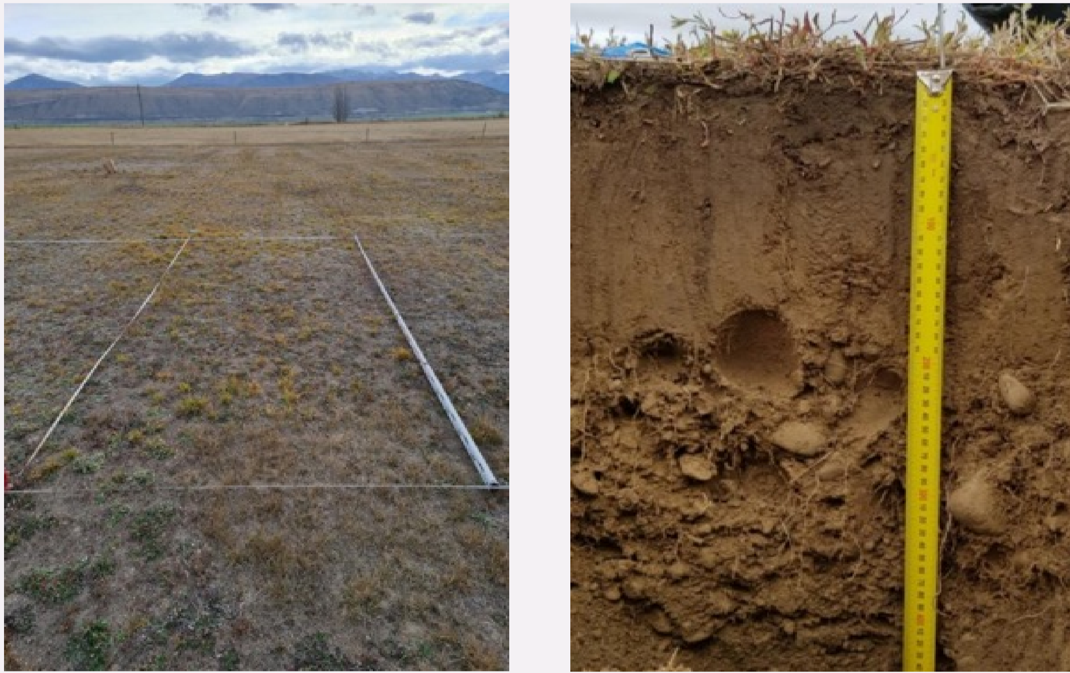
Figure 1: Native pasture on the surface (L), and shallow soil profile, depth to gravel is 20 cm (R) at the trial site.
